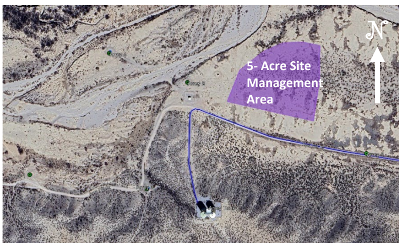
Fig. 1. The water treatment plant is located at ①. The purple area outlines the 5-acre reject-management site, the south-sloping land to the S and the dry river bed to the N-NW illustrate the geographical constraints for managing RO reject water.
